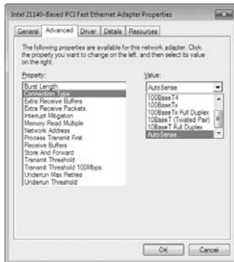
FIGURE 5.7 Advanced network interface properties
