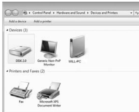
FIGURE 5.16 Devices And Printers with USB stick installed
